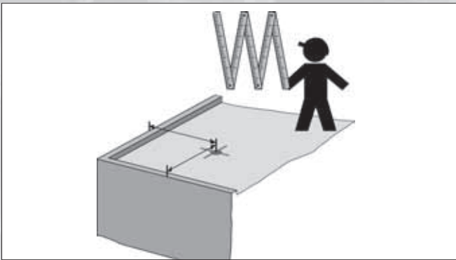
1. Measuring the position of the anchor point
