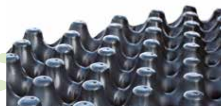
Floradrain® FD 25-E: Pressure-resistant, low drainage and water storage element made of recycled polyethylene for use in extensive green roofs.
