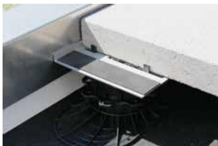
In the edge areas, the practical edge retainers ensure a stable position of the pavers without them wobbling. Thanks to the recesses in the edge retainers, the joint spacers on the support plate continue to ensure a uniform joint pattern here too.
