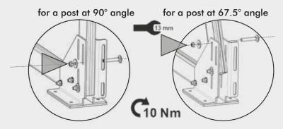
Fit washer and nut and tighten.
