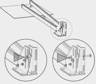
Loosen the marked nuts and remove the bolt.
