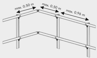
The distance from the joint to the post is max. 0.50 m on the one side, 0.50 m on the second side and then 0.96 m.
